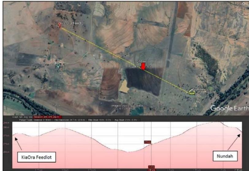
Figure 1: Elevation Profile between the Kia-Ora Feedlot and the Property 'Nundah'
