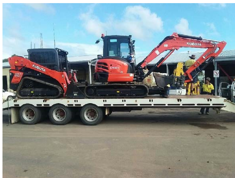
Mini Excavator and track loader on triaxle tag trailer.
